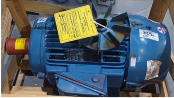
Electrical motor Sump pump Cu Cleaner Area.
